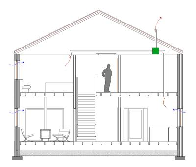
9.2 The total extract air flow rate during normal operation should be equivalent to at least 0.5 air changes per hour based on the volume of the whole dwelling. A facility to boost the air extract rate should be provided. It is preferable for a boost facility to target individual rooms rather than increase the overall extraction rate from the dwelling.
