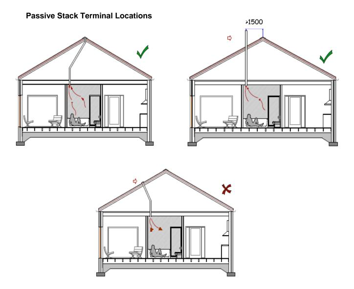
5.8 To minimise the resistance to air flow, ducts should consist of not more than one offset (i.e. not more than two bends) and these should be swept rather than sharp. Offsets should be no more than 45 degrees to the vertical.
