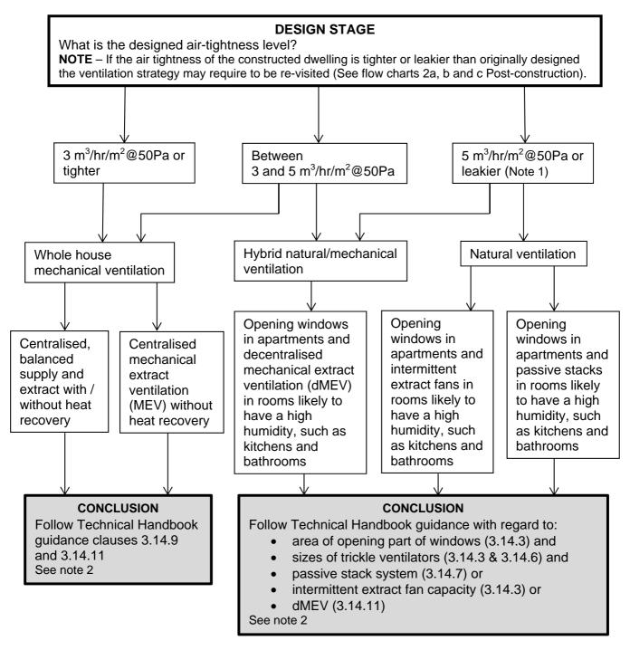
**Note 1**: Whole house mechanical ventilation is not generally suitable for dwellings with an air-tightness level leakier than  $5 \text{ m}^3/\text{hr/m}^2@50\text{Pa}$ .
